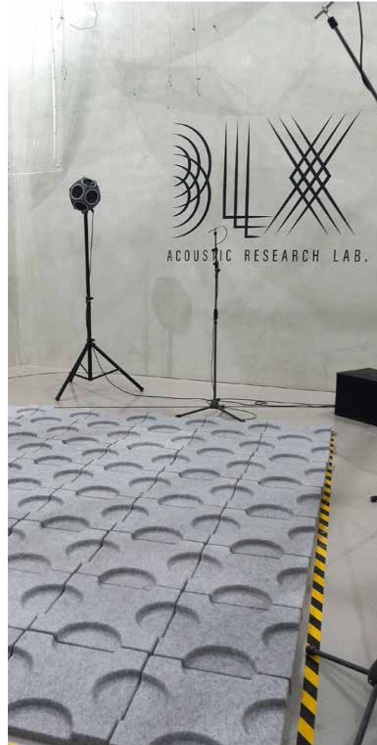
ISO 3741 is the standard for determining the sound power level of noise sources in a reverberation chamber by measuring sound pressure.
