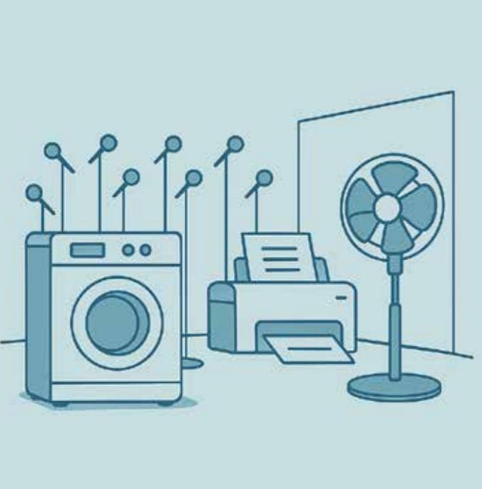
ISO 3743-2 describes the engineering method for determining the **sound power level of small and portable noise sources by measuring sound pressure in specially reverberant rooms**.
