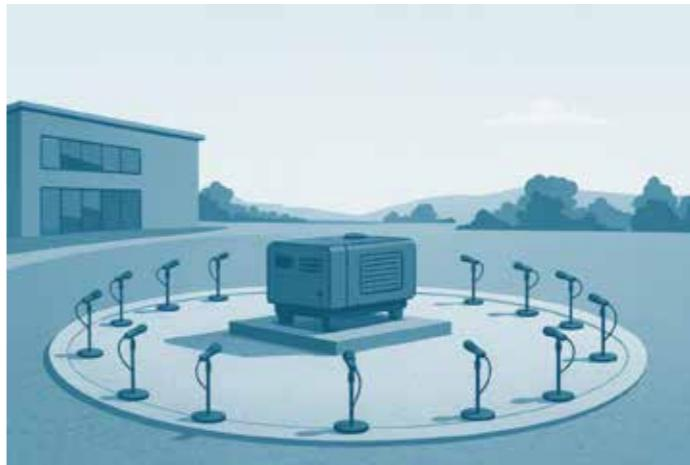
ISO 3744 is an engineering method **that determines the sound power level ( $L_w$ ,  $L_{wA}$ ) of noise sources by measuring sound pressure**.
