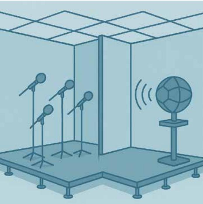
ISO 10848-2 is the standard that explains how to measure flanking (indirect) sound transmission between adjacent rooms for 'Type B' building elements.
