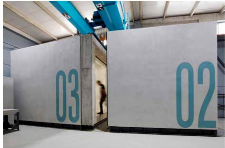
BLX ARL can perform measuring the airborne sound insulation of building products, such as walls, floors, doors, windows, shutters, façade elements, façades, glazing, small technical elements, for instance transfer air devices, airing panels (ventilation panels), outdoor air intakes, electrical raceways, transit sealing systems and combinations, for example walls or floors with linings, suspended ceilings, or floating floors.
